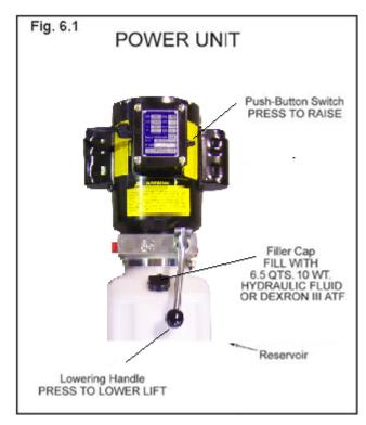
The standard power unit for your lift is 110 volt, 60HZ, single phase. All wiring must be performed by a certified electrician only. SEE WIRING INSTRUCTIONS AFFIXED TO MOTOR FOR PROPER WIRING INSTRUCTIONS.
