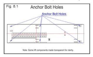
3. Using a 3/4" concrete bit, drill six holes on each pad 5" deep using the holes in the frame as a guide. (See Fig 8.2)
