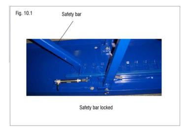
Check all MAIN SAFETY LOCKS to make sure they move freely and fall back to the lock position when released. Lubricate all SAFETY PIVOT points with WD-40 or equal. **KEEP HANDS AND FEET CLEAR**. Remove hands and feet from any moving parts. Keep feet clear of lift when lowering. Avoid pinch points.
