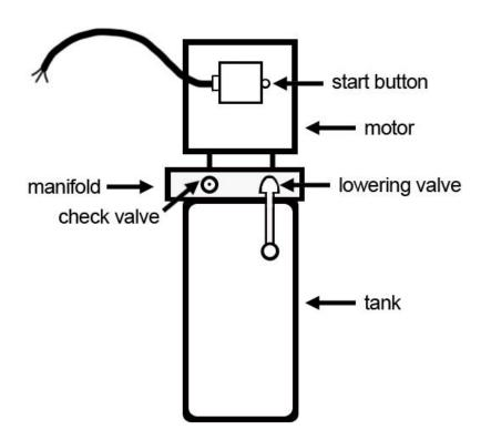
Step 2 – Using an Allen wrench and shop towel – with shop towel in place to catch fluid – loosen the check valve plug 2 ½ turns to allow it to leak.
