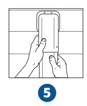
Complete the installation by attaching the top cover of the line guard into place making sure it clicks. Afterward, snap the rest of the pieces along the path to cover the remaining duct bases. Secure any unions or elbows using the included screws.
