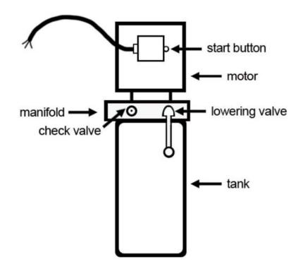
Step 2 – Using an Allen wrench and shop towel – with shop towel in place to catch fluid – loosen the check valve plug 2 ½ turns to allow it to leak.
