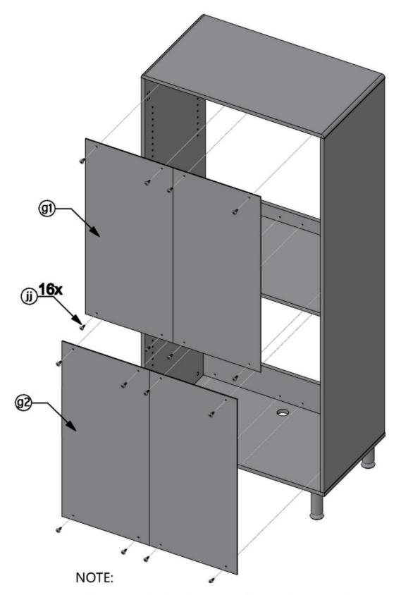
Align screw holes in Top Back Panel (g1) and Bottom Back Panel (g2) with screw holes in Back Spanners.
