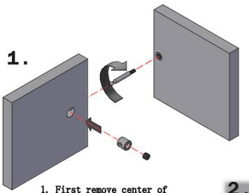
NOTE: After removing Cam(dd) screw, put in safe place. Make sure Cam is aligned as pictured and fully seated in hole. Test by inserting Metal Dowel(ee) into Cam. If Metal Dowel(ee) can't fully be insreted into Cam. pull out Cam and with flat head screwdriver, gently scrape away and loose wood and reinsert Cam properly aligned.
