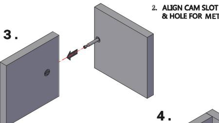
3. Install Metal Dowel (ee) into Cam outer ring before installing center of Cam into Cam outer ring(to prevent center of Cam blocking Dowel)
