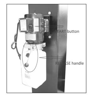
Fig. 15 start button & release button on motor
