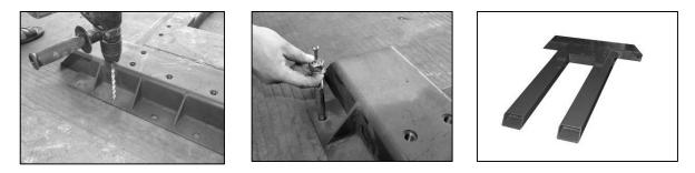
Fig. 3- A, B, C Anchoring the base plate
