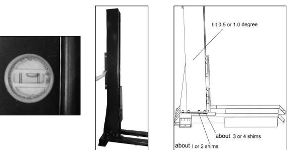
Fig. 5-A, B, C set up column (2)
