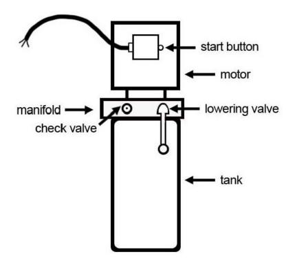
Step 2 – Using an Allen wrench and shop towel – with shop towel in place to catch fluid – loosen the check valve plug
